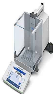
**The principle of operation** of these balances is based on the variations in the electrical characteristics of certain materials when they are subjected to mechanical compression.
