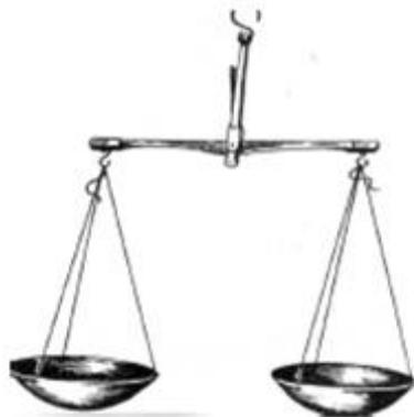
**It is used to weigh small amounts of substance, usually 0.05g-100-200g.**
