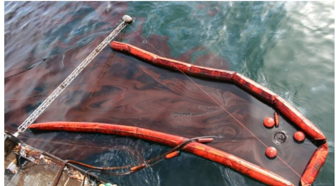
Skimmers come in various designs but all basically work by removing the oil layer from the surface of the water. (U.S. Coast Guard)
